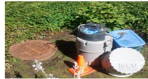
Figure 5: Isco-Autosampler installed at drain vault.
