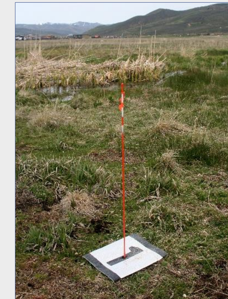
Right: Maggi Kraft records the exact GPS location of the control point. Left: A GPS control point which is visible in the IR imagery. Later used to georeferenced the image.
