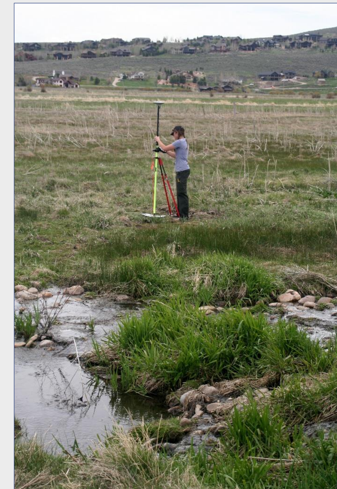
Right: Maggi Kraft records the exact GPS location of the control point. Left: A GPS control point which is visible in the IR imagery. Later used to georeferenced the image.
