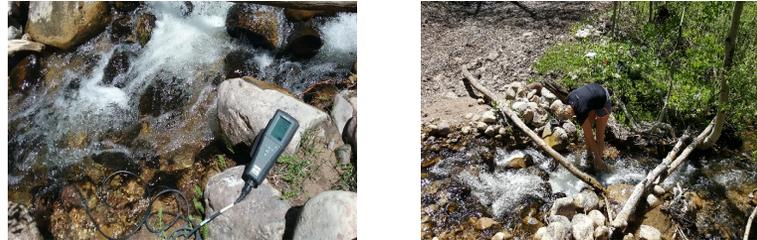
Figure 2. YSI probe used to measure temp, DO, and TDS (left) in use (right)
