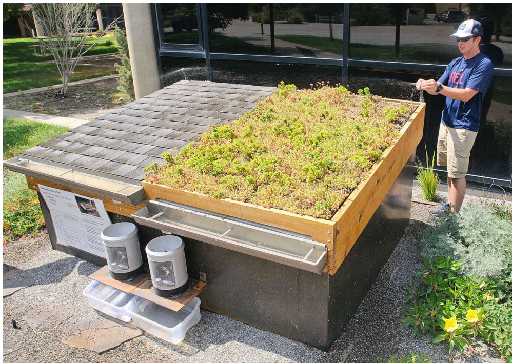
Cole Patton adjusts a sprinkler on a display that shows how water runoff is different for a roof with shingles vs. plants on Tuesday at USU.
