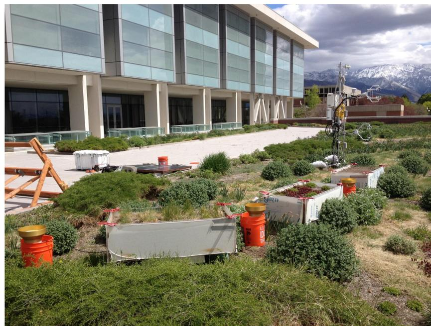
Figure 3. Three lysimeters used on Marriott Library green roof. From left to right: bluegrass, sedums, non-vegetated.
