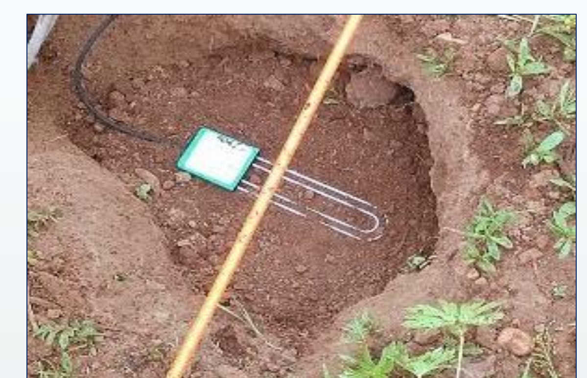
Fig. Acclima TDT sensor installation
