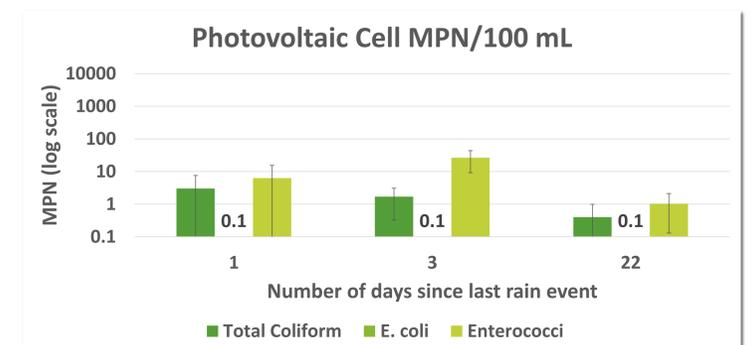
Figure 6. The average total coliform, *E. coli*, and enterococci for the photovoltaic cell.
