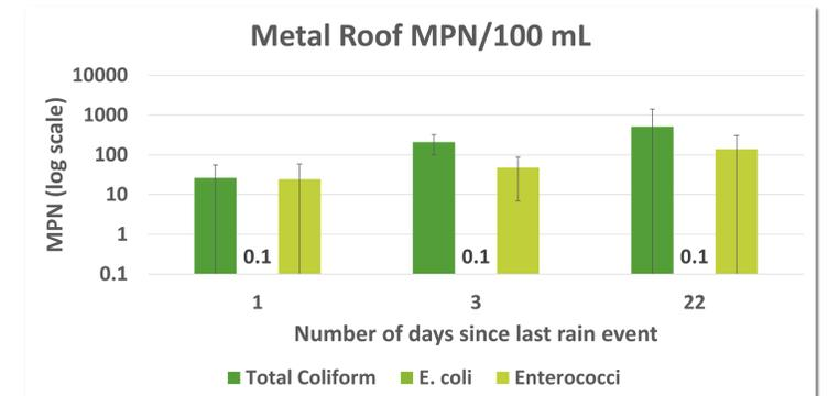
Figure 5. The average total coliform, *E. coli*, and enterococci for the metal roof.
