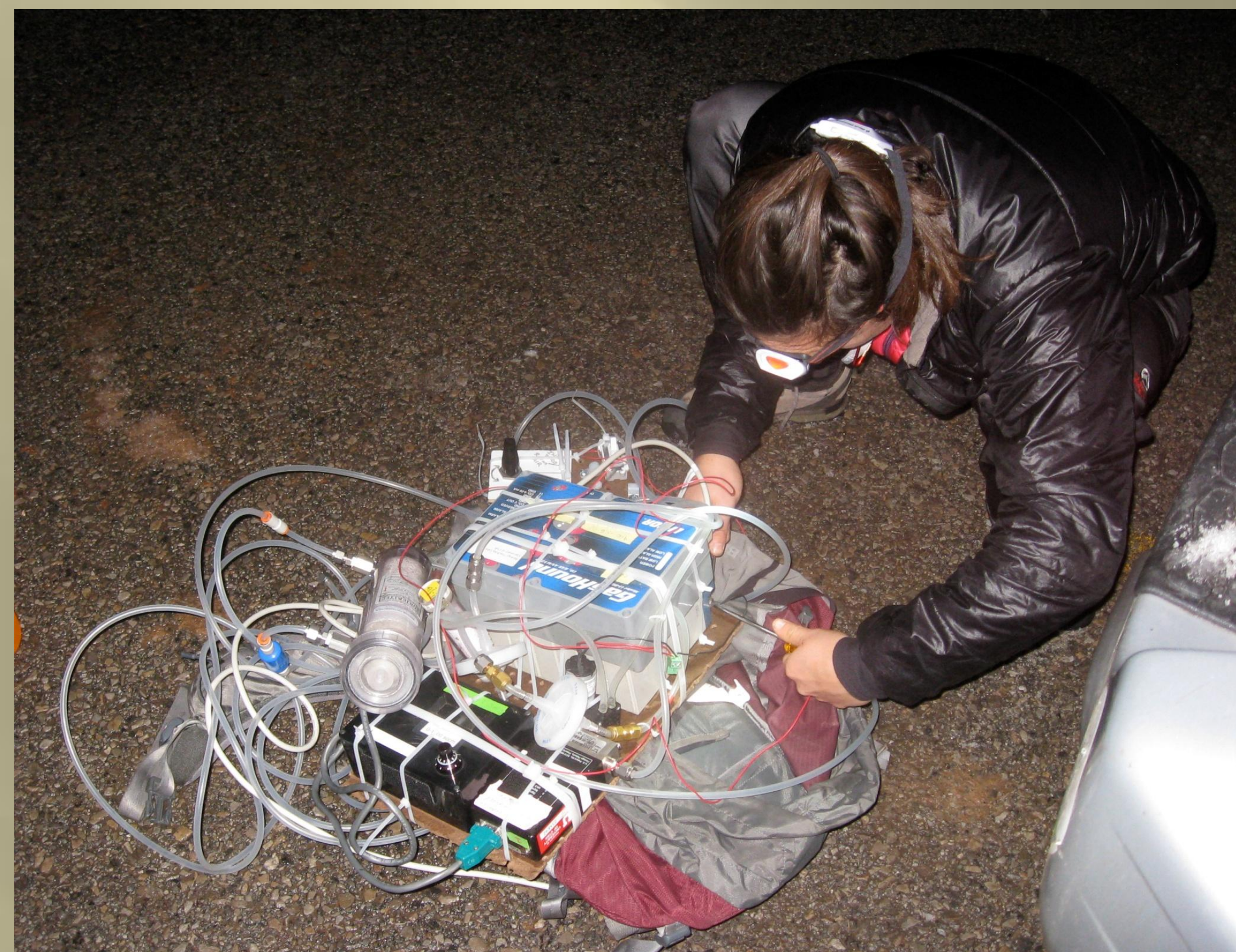
Figure 2. Assembling portable field equipment for a quasi-vertical human-powered CO 2 transect.
