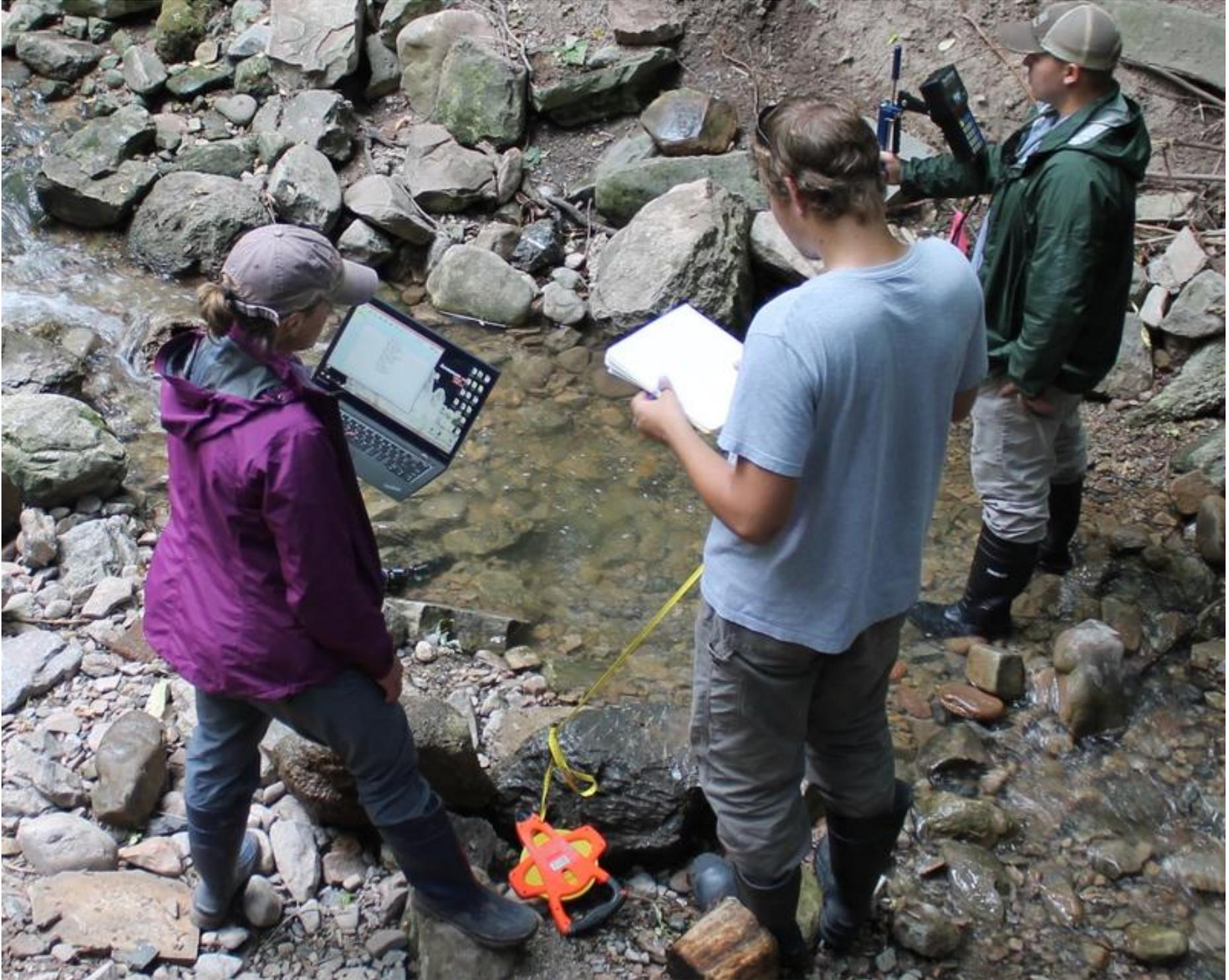
*This team from Utah State University is measuring how much water is flowing in Red Butte Creek at this location. They are part of the collaborative effort to gain an in-depth understanding of how western streams work.*
